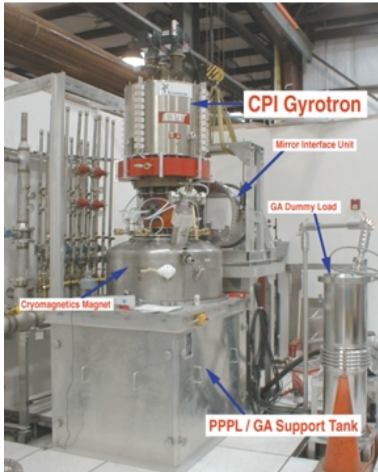
FIGURE 2.2 A gyrotron from the DIII-D tokamak experiment at General Atomics (GA) in San Diego. A gyrotron is a source of high-frequency radio waves for heating electrons. Courtesy of General Atomics.
