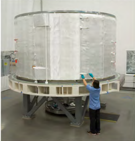
FIGURE 2.8 (a) Ground insulation being applied to a central solenoid superconducting module at General Atomics (Poway, CA). The insulation must be precisely placed and consists of 18 layers of fiberglass, six layers of Kapton sheets totaling over 2,300 square meters, and a ground plane. (b) The ITER central solenoid will consist of six stacked modules, stand nearly 18 meters tall, and weigh more than 900 tons. When completed, it will be the largest pulsed superconducting magnet in the world.
