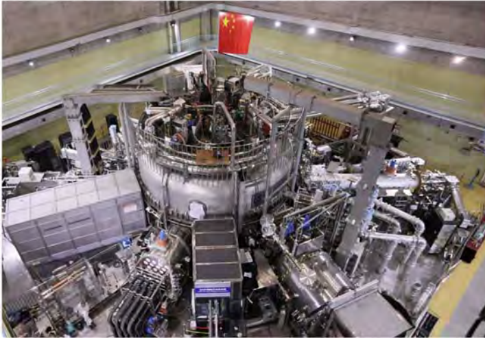
FIGURE G.3 Experimental Advanced Superconducting Tokamak (EAST) is a superconducting tokamak demonstrating high-fusion confinement performance in steady-state. EAST has a major radius of 1.8 m, and the EAST superconducting magnets are energized to 320 MJ. See http://english.ipp.cas.cn/rh/east/ .
