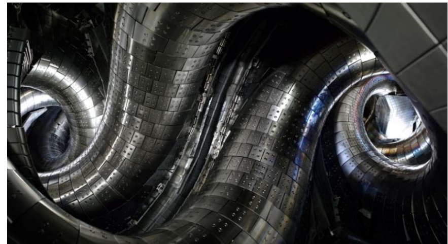
Inside the vacuum vessel (LHD)
