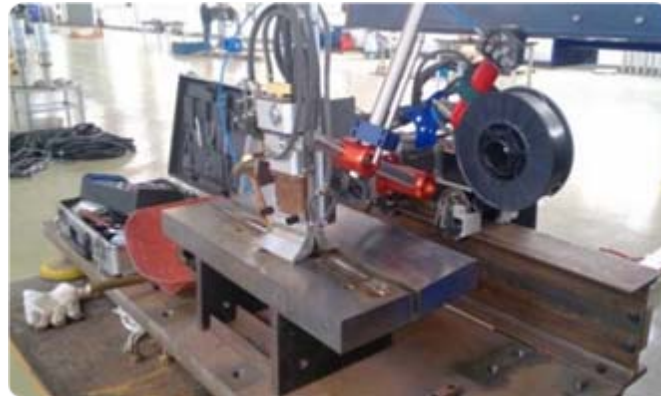
R&D of Narrow Gap TIG Welding on VV
