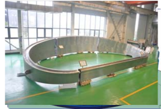
Assembly of VV Poloidal Sectors
