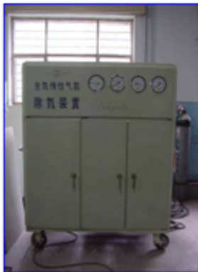
D.S. for inert gas Metallic getter approach
