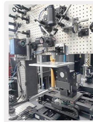
a GA-BUILT GEN-2 2PP SYSTEM
