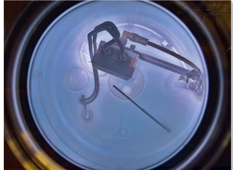
Vacuum Chamber Installed – Mirror Cleaning Facility at PPPL First plasma produced to prototype mirror cleaning methodology
