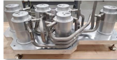
Antenna Block Assembly Water Circuit Welding Trial
