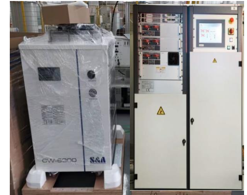
Chiller and C&C Cabinet
