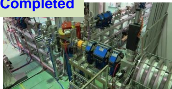
D-T Neutron Generator HINEG-Ia in Hefei ( 6.4 \times 10^{12} n/s)
