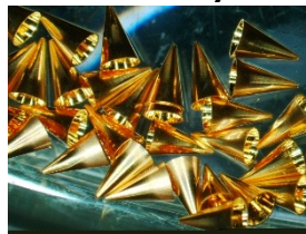
Cone-in-shell targets assembled with \pm 10 \mu\text{m} accuracy
