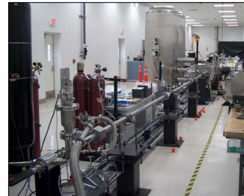
Gas gun with sabot: 400 m/s with 0.59 mrad accuracy, 50 m/s with mrad accuracy 0.24
