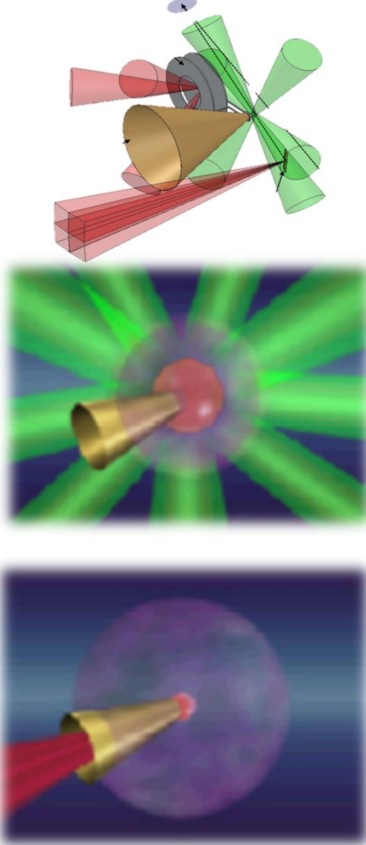
The isochoric heating of the compressed core [1] was improved by collimation of the REB with kilo tesla magnetic field generated by power laser[2].
